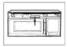
Next, remove the single screw located above door near center of oven that secures light housing. Remove bulb and replace with a 30-watt GE bulb (Part No. WB2X4235) available from your GE supplier. Secure light housing with screw.
